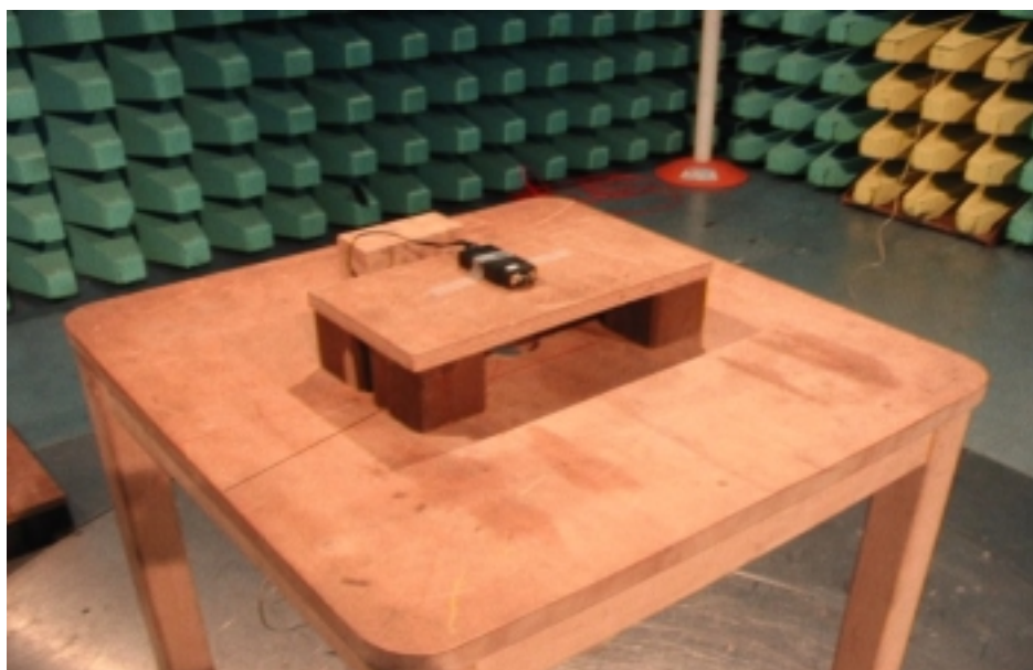
View during the radiated emission measurement
