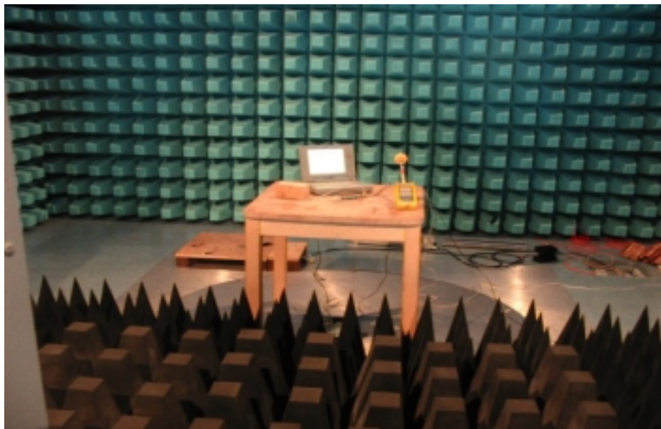
View during the radiated emission measurement
